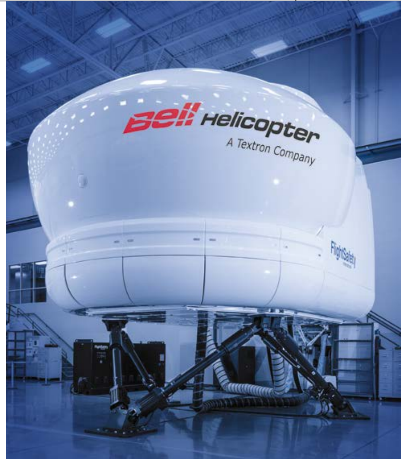
FlightSafety's new FS1000 Level D qualified full flight simulator.
